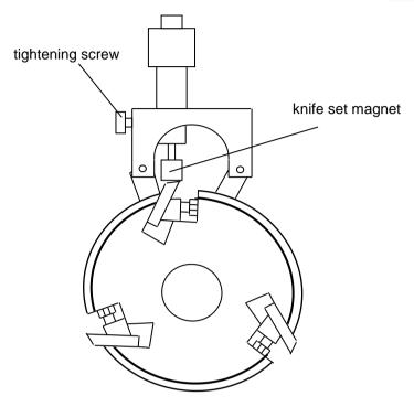
**Adjustment:** Bring the knife set magnet into the desired height by turning the adjus Read off the scale the position. When having reached, tighten with the tightening sc
