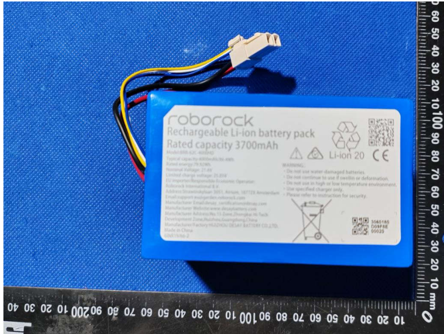
电池组外观 1 View of the battery 1
