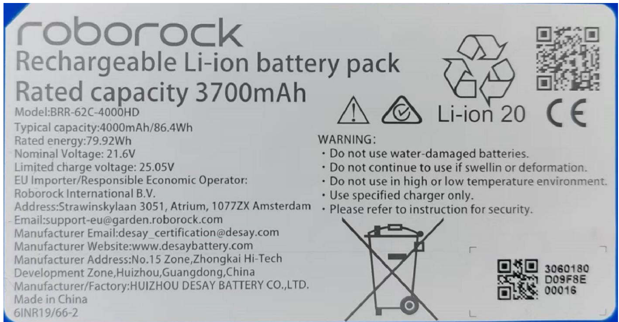
电池组铭牌 View of the battery name
